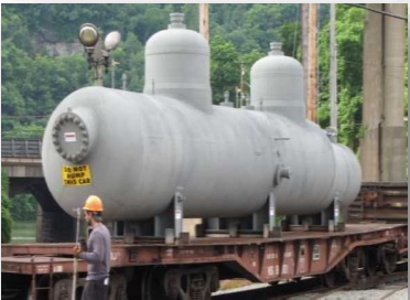
Horizontal Steam Generator
