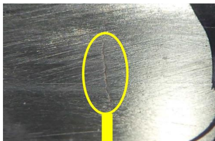
傷の長さ:2.0 mm (研磨後)
