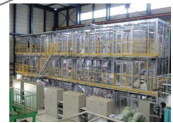
H 2 production test facility (0.1 m 3 /h)
