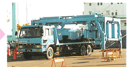
Radioactivity measurement is made by the gate monitor.
