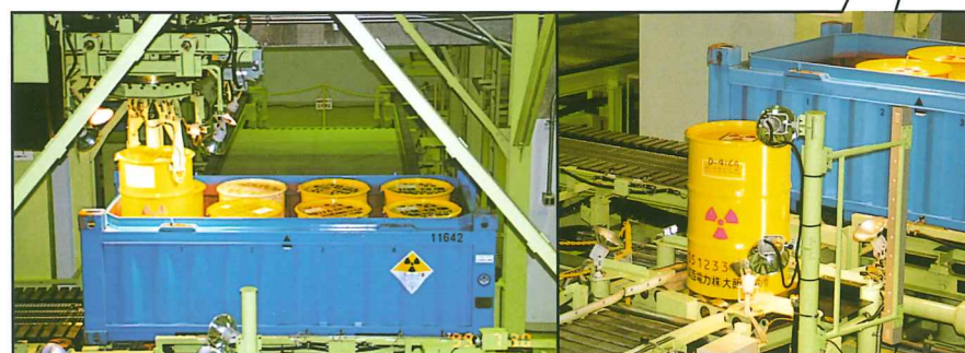
Waste packages raised to inspection device
