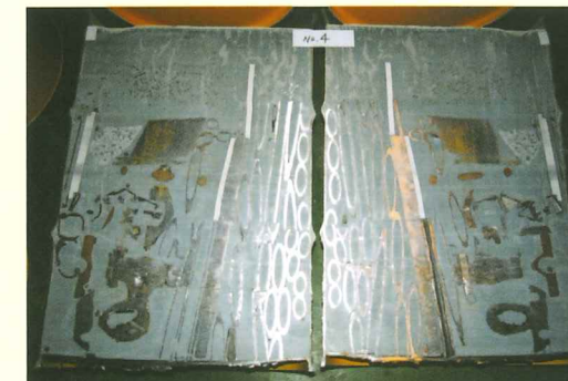
Metal stored and solidified with mortar
