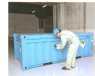
Surface inspections are made of the radioactivity dose rate before the waste is transported.
