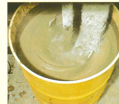
Concentrated waste solidified with cement
