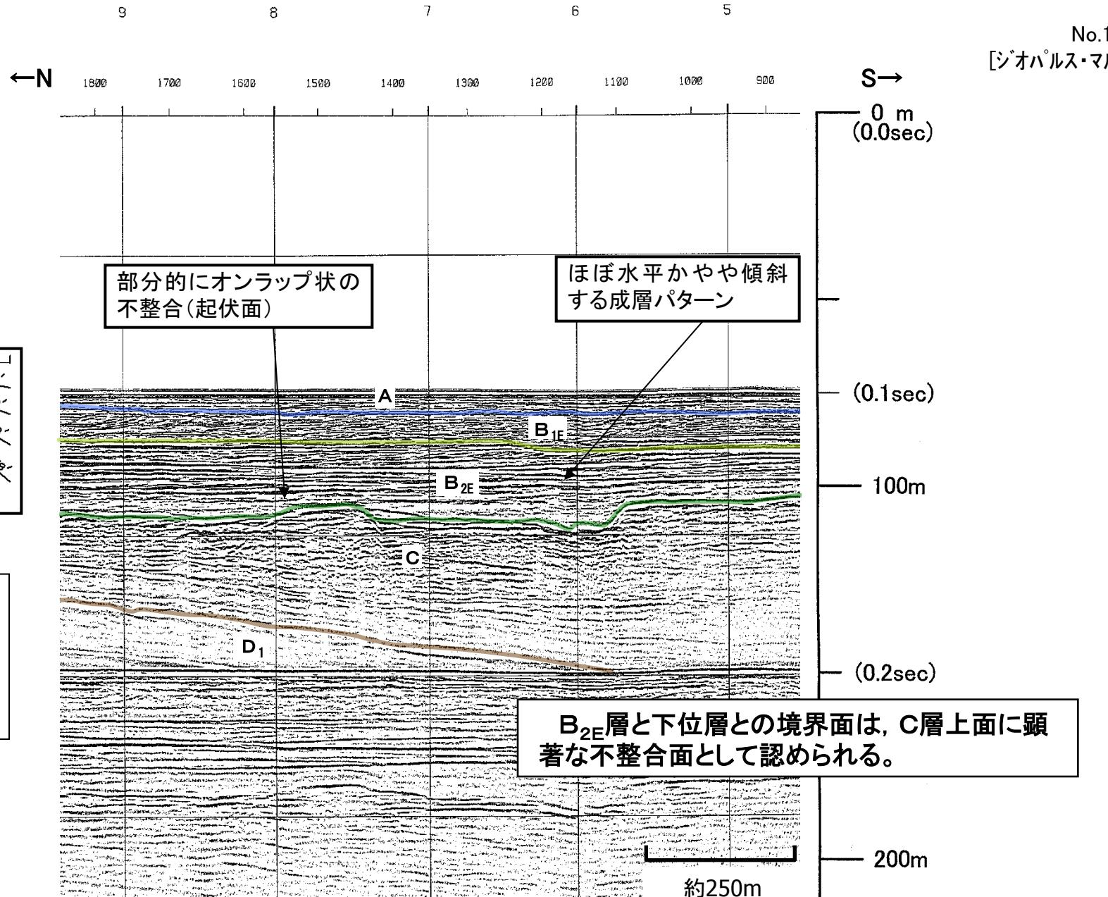
**B<sub>1E</sub>層とB<sub>2E</sub>層の不整合面の分布(東部海域)**
