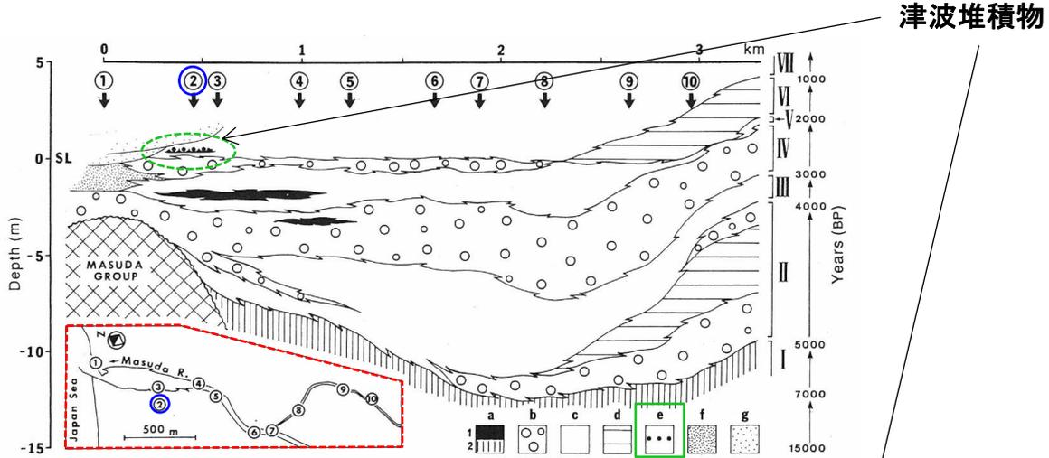
Fig. 2 Lateral and vertical distribution of sedimentary sequences of the Masuda Plain (Fig. 1). The section is based on numerous borehole data 1-10. Borehole sites, a-g: sedimentary environments (a-1: fresh-water lagoon, a-2: brackish lagoon, b: fluvial channel, c: flood plain, d: abandoned river, e: tsunami deposit, f: beach, g: dune), I-VII: transgressive-regressive facies (I, III, V and VII: transgressive facies; II, IV and VI: regressive facies). SL: Present high water mark.
