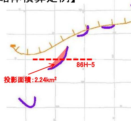
$$100\text{m}(\text{厚さ}) \times 2.24\text{km}^2(\text{投影面積}) = 0.22\text{km}^3$$
