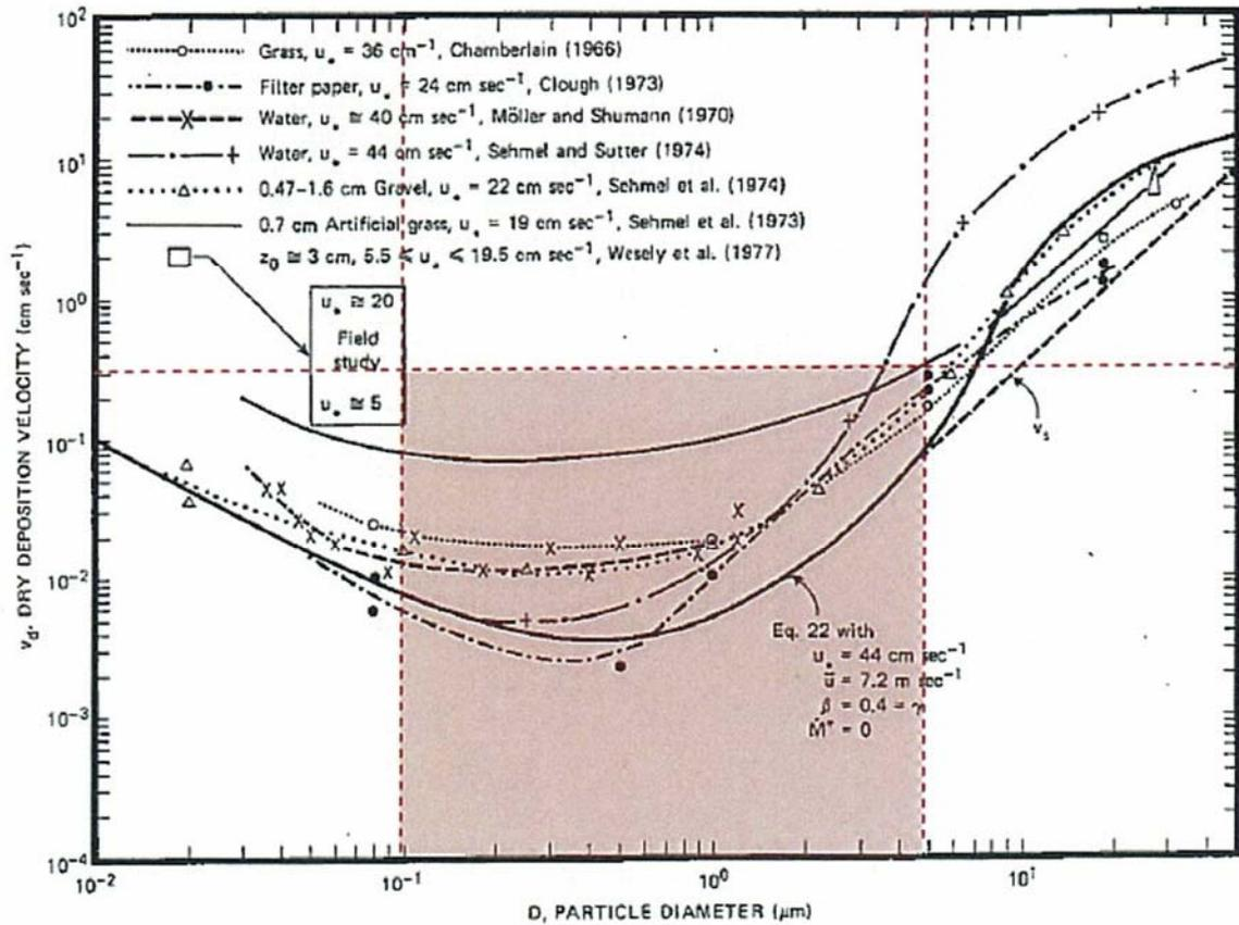
Fig. 4 Dry deposition velocity as a function of particle size. Data were obtained from a number of publications.<sup>1, 2, 3, 4</sup> The theoretical curve appropriate for a smooth surface is shown for comparison. Note that the theoretical curve is strongly dependent on the value for  $u_*$  and that Eq. 22 does not contain a parameterization for surface roughness. For a preliminary study of the effect of surface roughness and other factors, see Ref. 5.
