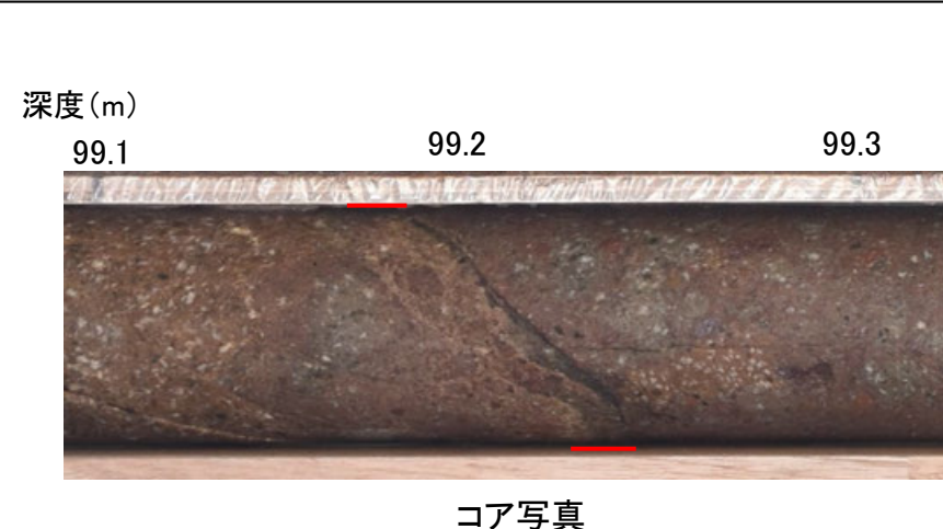
⑬深度99.19～99.22mに厚さ2.5cmの破砕部(N5E/61SE)
