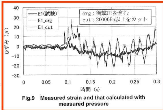
Fig.9 Measured strain and that calculated with measured pressure
