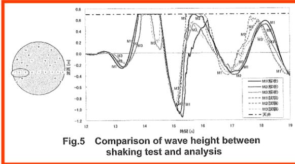
Fig.5 Comparison of wave height between shaking test and analysis
