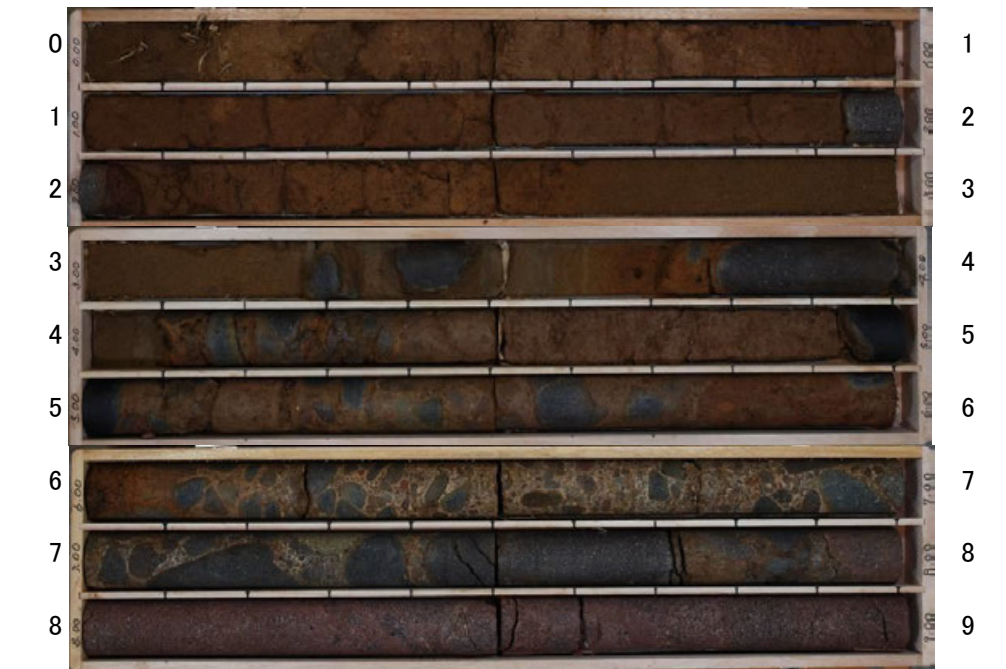
Site 5 (孔口標高48.84m, 掘進長9m, 鉛直)
