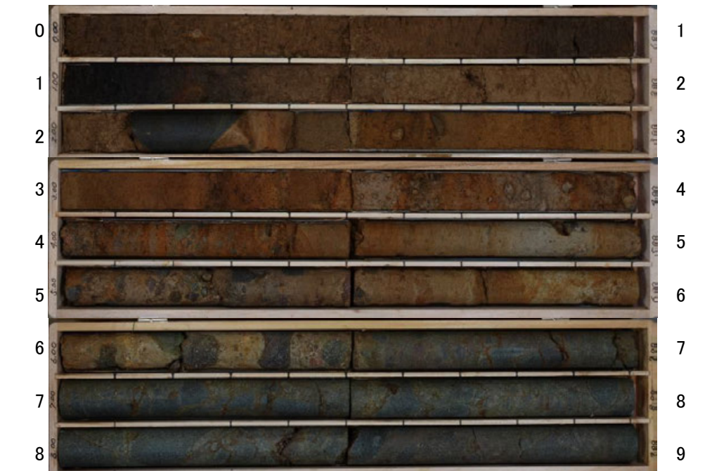
US-N04(孔口標高45.04m, 掘進長9m, 鉛直)
