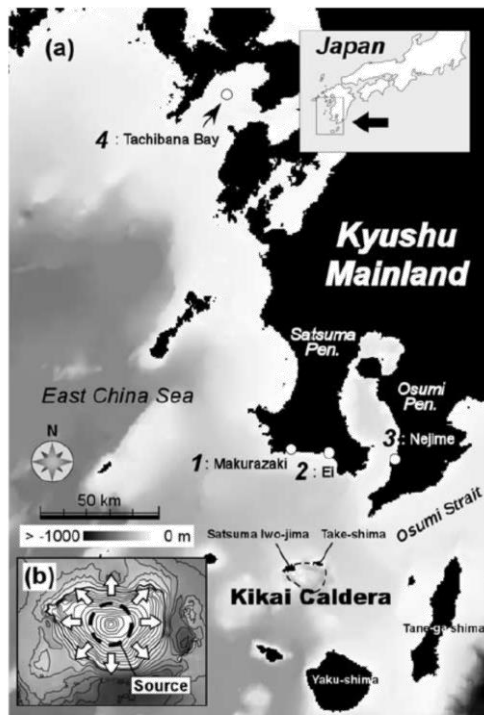
Figure 1. (a) Location of the Kikai caldera, south of Kyushu, Japan. This map also shows the computed area used for the numerical simulations. Tsunami data were collected at four points (1: Makurazaki, 2: Ei, 3: Nejime, 4: Tachibana Bay). (b) In the numerical simulations, pyroclastic flows are generated from a circular source of 4 km radius in the center of the pre-caldera island.
