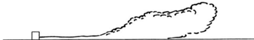
Fig. 3. Dispersion of vapor cloud of the cryogenic liquefied gas
