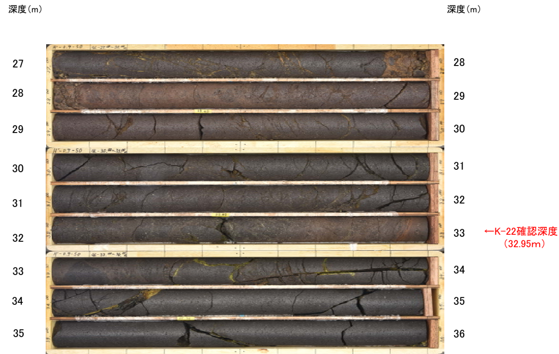
H'-0.9-50孔(掘進長40.00m, 傾斜50°)
