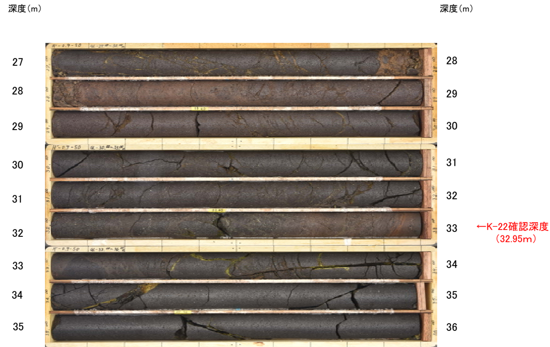
H'-0.9-50孔(掘進長40.00m, 傾斜50°)
