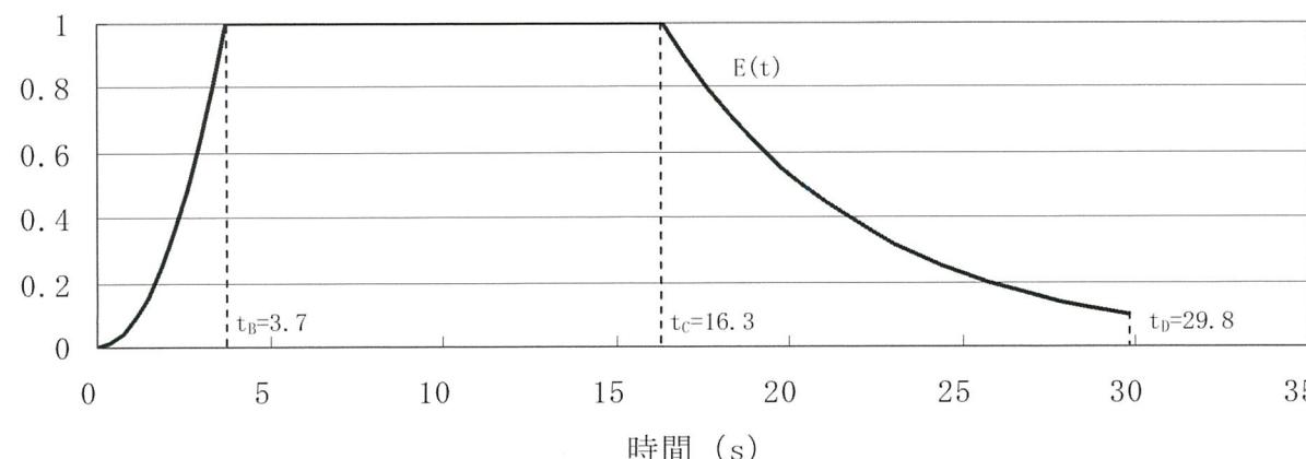
$$E(t) = \begin{cases} (t/t_B)^2 & (0 < t \leq t_B) \\ 1.0 & (t_B < t \leq t_C) \\ e^{\frac{\ln(0.1)}{t_D - t_C}(t - t_C)} & (t_C < t \leq t_D) \end{cases}$$
