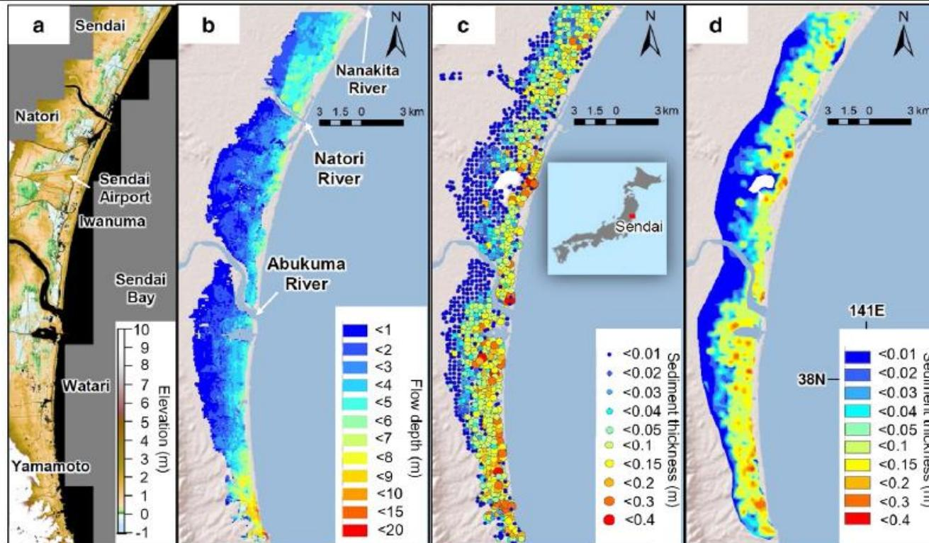
Fig. 1. (a) Topographic map at Sendai Plain (post-tsunami 5 m DEM data). (b) Interpolated flow depth data (m) of 100 m grid. (c) Sediment thickness data (m) obtained from Miyagi Prefecture/Midori-net Miyagi. (d) Interpolated sediment thickness data (cm) for a 50 m grid.
