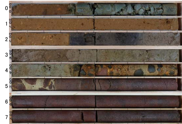
US-N07(孔口標高43.47m, 掘進長8m, 鉛直)
