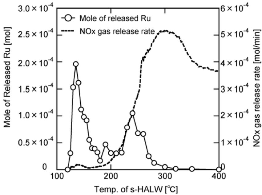
Fig. 7 Comparison of released amount of Ru with NO<sub>x</sub> gas release rate
