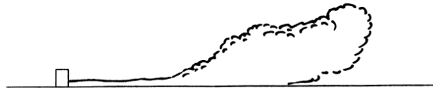
Fig. 3. Dispersion of vapor cloud of the cryogenic liquefied gas
